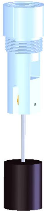
The model valve 47-20 is pre-assembled for installation with a 12" x 1/4-20 threaded rod. The threaded rod should be cut to determine a Length L as shown in Figure 1. This length L will determine the fill capacity for shut off as specified by the tank specification manual for 90% or 95% capacity.
